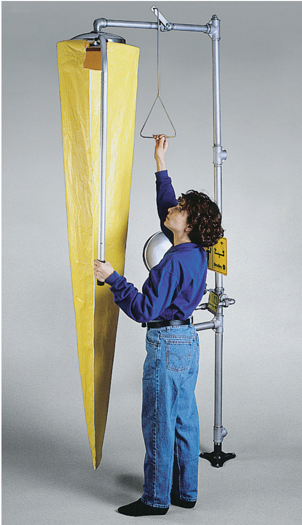
A heavy-duty tester provides a convenient way of testing drench showers to comply with ANSI specifications for weekly testing – without getting wet. The watertight funnel has a weighted bottom and directs water to a drain or bucket.
