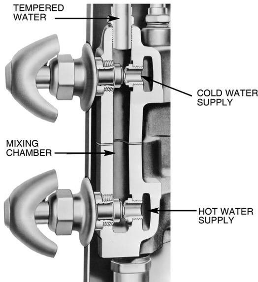
The hot supply to these valves should always be tempered by a master controller, either at a remote location or mounted in the shower equipment.
