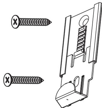
**NOTE:** Small slot in the clip allows for added adjustment when using more than two clips to hold weight on an extra large mirror.
