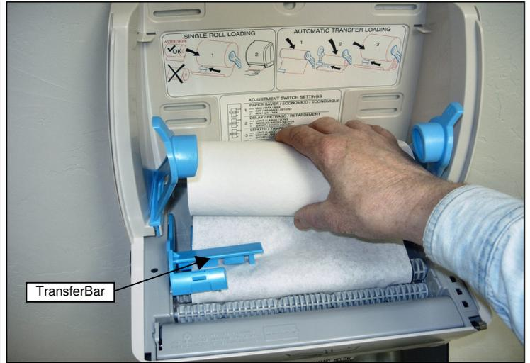
2) Carefully remove the stub roll, making sure the paper web is under the transfer bar.
