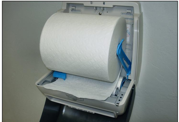
4) Install a new roll with the web coming off the back. Place tail of paper under transfer bar.
