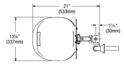
All dimensions assume standard thread engagement. Variations in manufacturing allow for +/- ½ (3mm) per threaded joint. To find the tolerance of a dimension, add the number of thread joints across the length of the dimension and multiply it by ½ (3mm).
