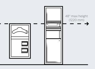
In order to create a safe environment for visually impaired patrons, fixtures must be detectable with a cane. The diagram above highlights this requirement.
