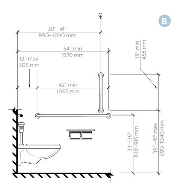
Dimensions are shown for grab bars installed with protruding or recessed dispensers.
