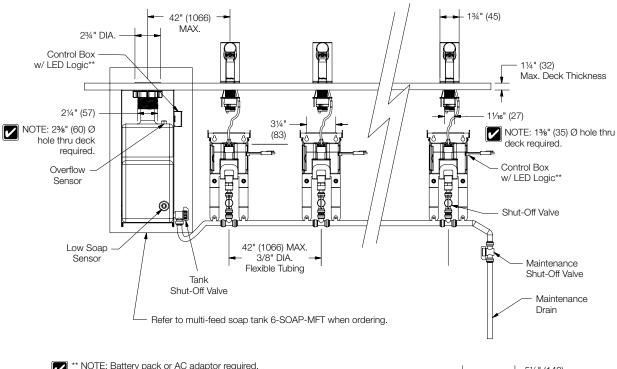
\*\* NOTE: Battery pack or AC adaptor required. AC power source required to be within 54" (1371) of the control box.
