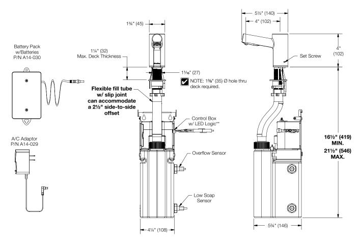
\*\* NOTE: Battery pack or AC adaptor required. AC power source required to be within 54" (1371) of the control box.
