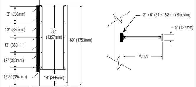
Generally recommended for Sight Screen application. Screen has floor mounting and requires minimum 3" concrete floor for anchoring.
