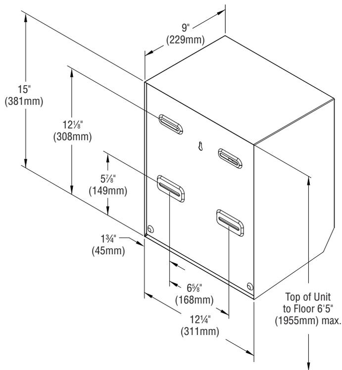
**⚠ IMPORTANT:** For unobstructed forward or side reach, the unit should be installed so that the top edge of dispensing area is 48" (1219mm) maximum above finished floor (AFF).
