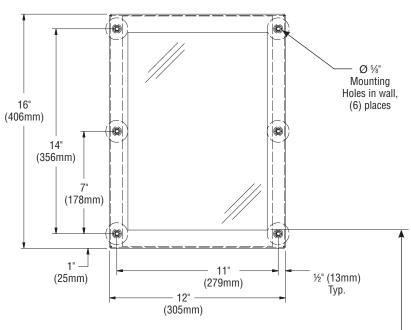
IMPORTANT: For compliance with ADA accessibility — guidelines, the bottom edge of the reflecting surface should be installed 40" (1016mm) maximum above finished floor.
