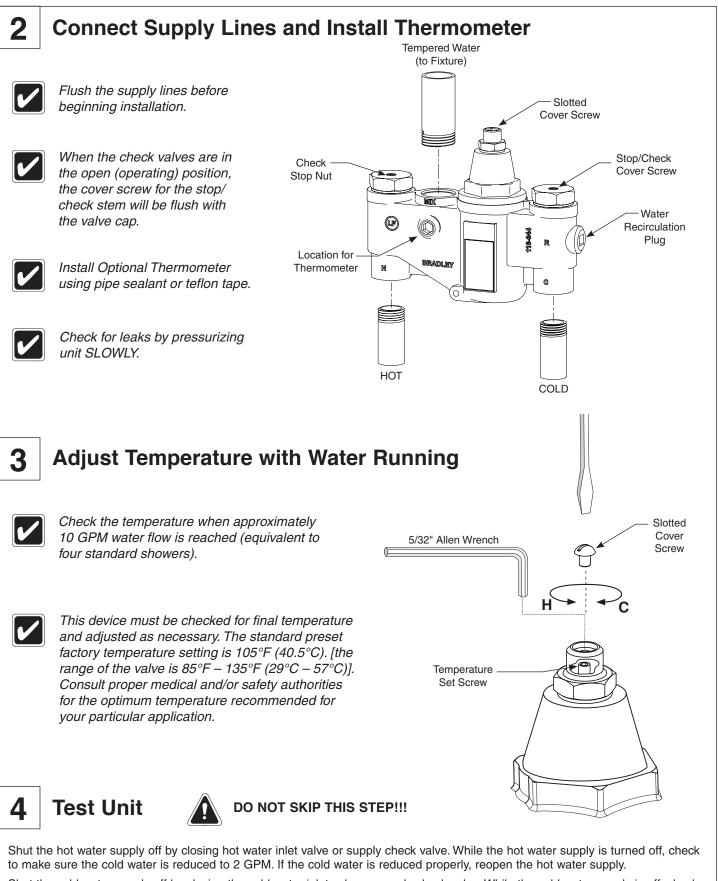
Shut the cold water supply off by closing the cold water inlet valve or supply check valve. While the cold water supply is off, check to make sure that the hot water flow has shut down. If hot water is shut down, reopen cold water supply. Test unit weekly for proper function and desired set temperature.
